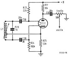
Fig. 7 - Oscillatore 100 kHz submarker.
